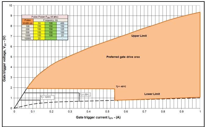
**Fig14 Gate Characteristics**
