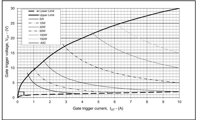
Fig. 15 Gate characteristics
