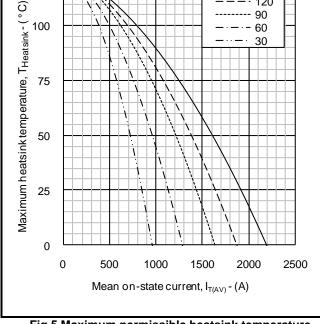
Fig.5 Maximum permissible heatsink temperature, double side cooled - sine wave
